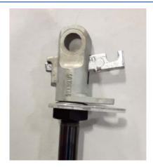
4 Holding the pin in place screw the cylinder, with cable clip assembly, into the actuator. Make sure the pin stays in place at all times. Tighten the actuator on the cylinder until the pin reaches the top of the hole in the actuator. Do not over tighten.
